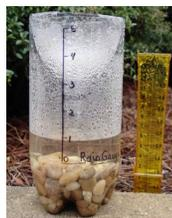
When it rains, monitor your rain gauge. Measure & record # inches/hour. Be sure to empty your gauge after each reading.
